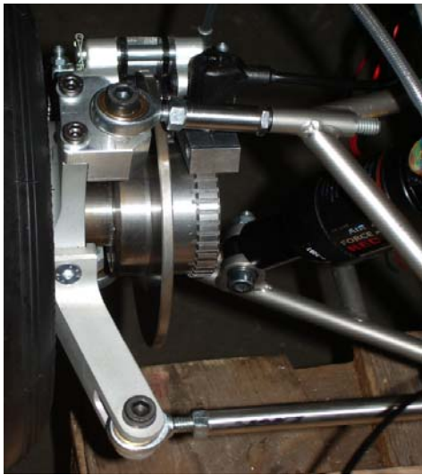
Figure 9: Kart 1, increment- and brake discs
