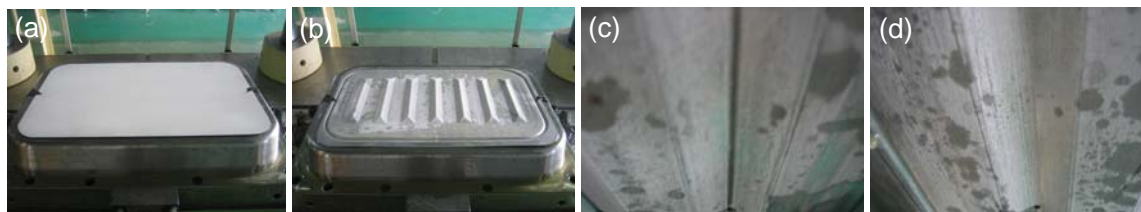
Figure 6. (a) Al sheet before hydroforming, (b) Al sheet after hydroforming, (c) 1mm radius profile after hydroforming, and (d) 7mm radius profile after hydroforming
