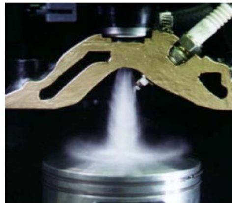
Figure 7: Fuel Spray from an Orbital Air-Assisted Fuel Injector [3]
