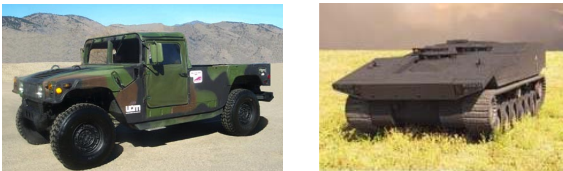
Fig. 6. Hybrid Electric HMMWV (14) and Future Combat System-Tracked prototype FCS-t (15)
