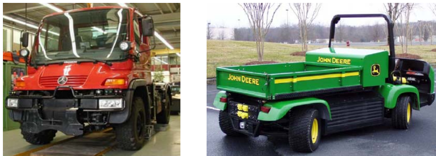
Fig. 5. DaimlerChrysler Unimog UGN E-Drive (7) and John Deere Fuel Cell Hybrid CWV (Commercial Work Vehicle) (14)
