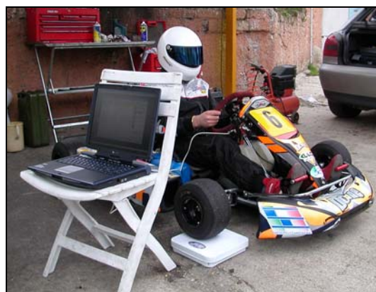
Figure 6: Static test for load transfers
