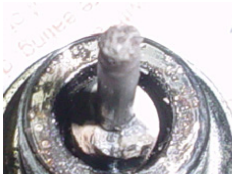
Fig. 6. A central electrode broken after activity
