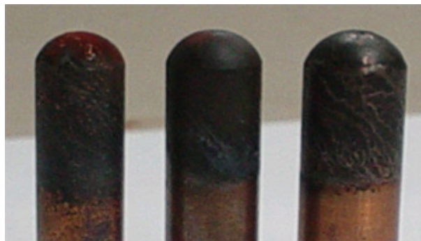
Fig. 8. Central copper electrodes(From left to right, diameter 10, 11 and 12 mm)
