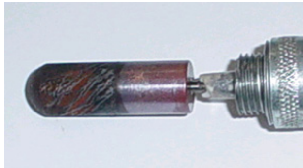
Fig. 7. A central copper electrode after 60 minutes of activity
